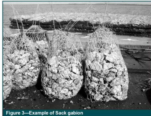
Figure 3—Example of Sack gabion
